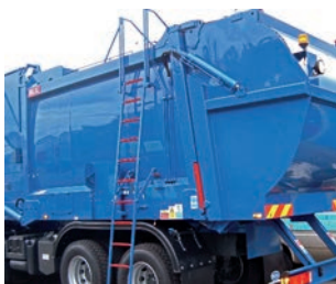
Roof Access Ladder
